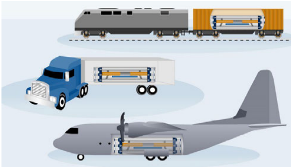
Figure 11. Examples of microreactor transportation options 50
